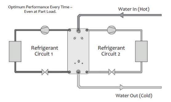
ClimaCool modular chillers employ reliable and highly efficient brazed plate heat exchangers. These compact exchangers are true dual-circuit heat exchangers in which each water channel is flanked by two refrigerant circuits. This design gives maximum performance, even at part-load.
