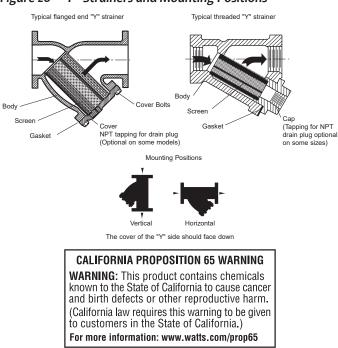
Figure 28 - "Y" Strainers and Mounting Positions
