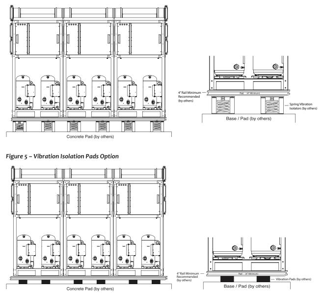
NOTE: Size and weight distribution is to be determined by a qualified structural engineer per individual job requirements.
