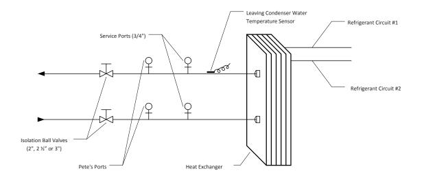
Figure 18 - Chilled Water Circuit
