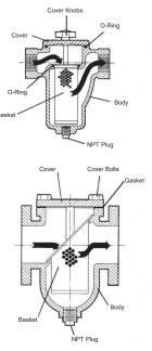
Basket Strainers should be installed in the position shown in the illustrations above.
