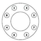
NOTE: Excessive bolt torque may damage flanges. Please refer to established flange bolt torques for guidelines.
