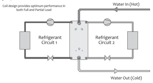
ClimaCool modular chillers employ reliable and highly efficient brazed plate heat exchangers. These compact exchangers are true dual-circuit heat exchangers in which each water channel is flanked by two refrigerant circuits. This design gives maximum performance, even at part-load.
