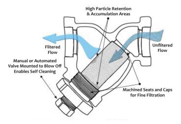
Figure 35: WYE Strainer - Flanged Ends
