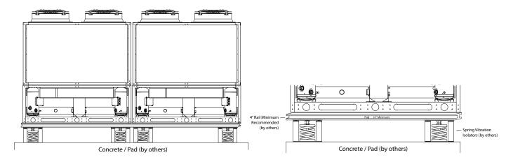
Figure 12 - Vibration Isolation Pads Option
