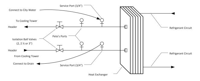
Figure 26 - In Place Cleaning Arrangement
