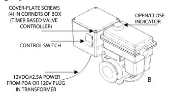
Figure 32 - Valve Specifications
