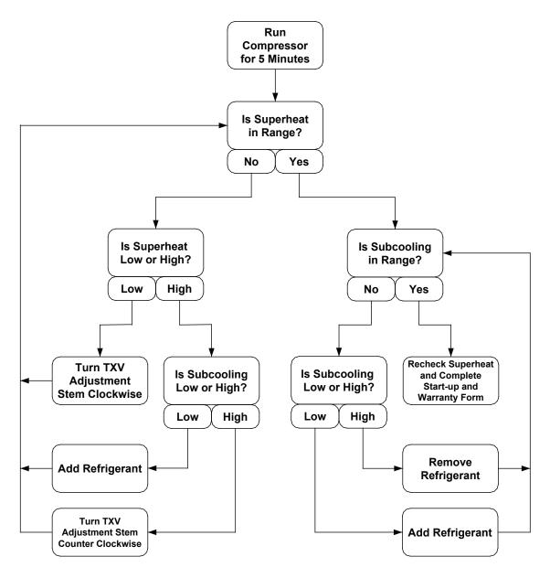
CAUTION: Do not charge to achieve subcooling temperature when the expansion valve is overfeeding. If the expansion valve is overfeeding, readings may still indicate low subcooling and low superheat, but circuit may not be undercharged.
