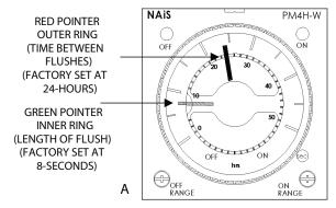
Figure 31 - Electric Ball Valve
