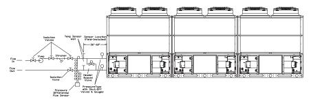
Figure 21 - Field Piping Reverse Return - (Preferred 1 to 5 modules) Required for 6 or more modules
