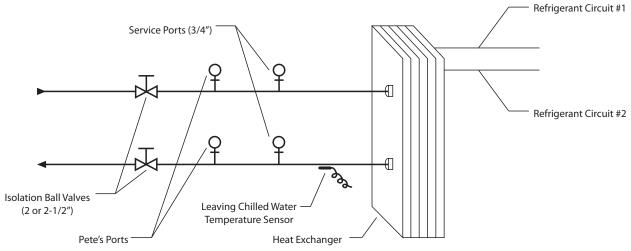
**NOTE:** Figure 22 depicts hydronic piping in each ClimaCool chiller module and is shown with water isolation valves.
