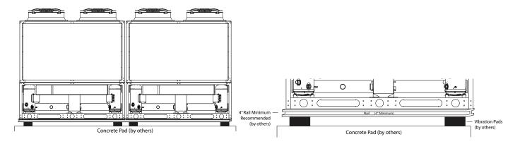
**NOTE:** Size and weight distribution is to be determined by a qualified structural engineer per individual job requirements
