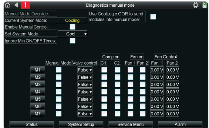
**Current System Mode:** Displays the current manual mode.
