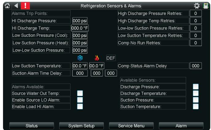
**HI Discharge Pressure:** Sets the threshold above which the DISCHARGE PRESSURE ALARM is triggered for the selected refrigerant.
