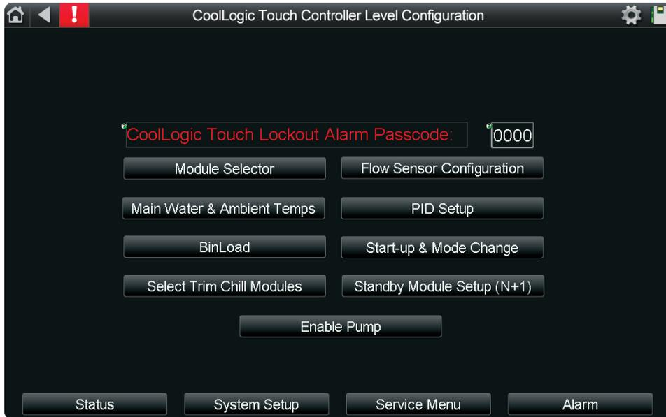
**CoolLogic Touch Lockout Alarm Enter Passcode:** The required Passcode to unlock the unit.
