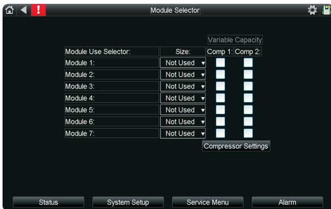
**Module Size Options are:** Not Used, 20 Ton, 30 Ton, UCF 20/30, 50 Ton, 70 Ton, 85 Ton, UCF 50/70.
