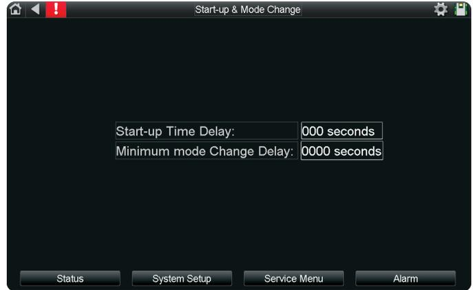
**Start-up Time Delay:** The time delay before the unit starts up.
