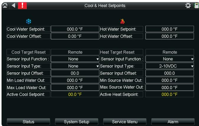
Under **Local**, select Hot (or Cool) water setpoint and enter the desired setpoint for each mode. The Min/Max for Load/Source Out is for bank safeties where a breach in these values disables the unit from running.
