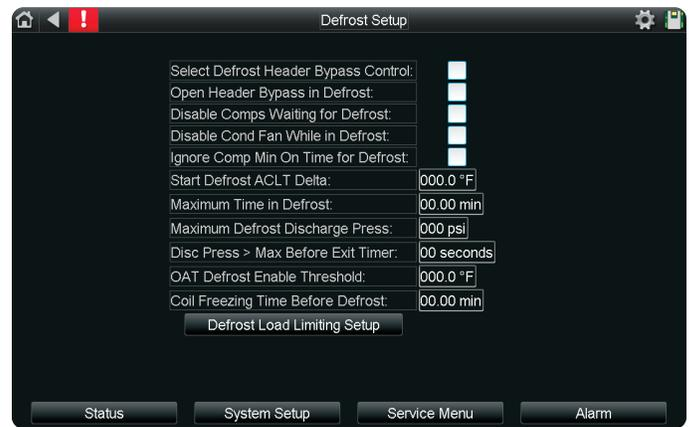
**Select Defrost Header Bypass Control:** The Header Bypass is locked open in defrost if this is enabled with 'Open Header Bypass in Defrost'.
