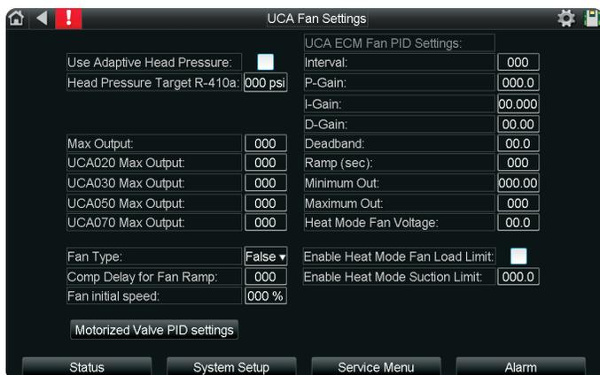
**Use Adaptive Head Pressure:** Uses a custom curve to match appropriate head pressure to ambient temp (not recommended).
