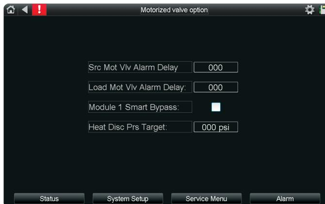
**Alarm Delay:** The delay between the valve open command and valve feedback before an alarm is triggered.
