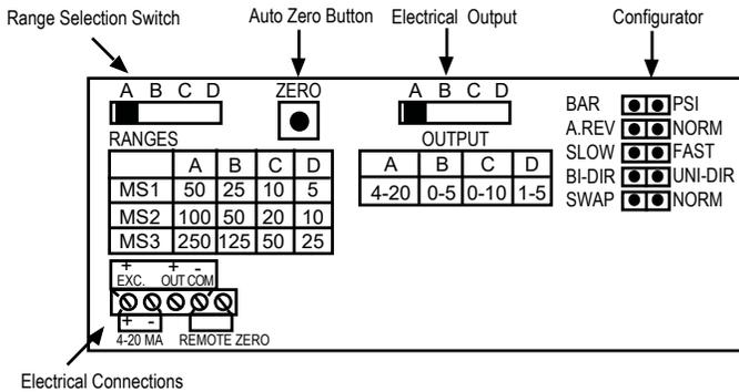
Calibrate the DPTs while the tubing is connected to the appropriate piping and the pump is not running. The pressure differential should read 0.0. If not, confirm that the tubing is properly connected, the pumps are off, the DPT is wired correctly, and there is no air in the lines. Adjust as needed using the OFFSET fields shown in the *Flow Sensor Configuration Screen*.
