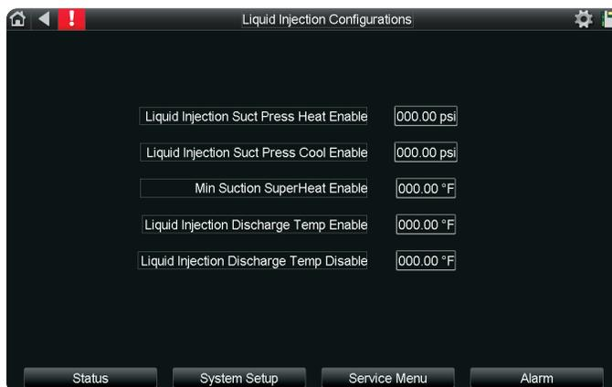
**Liquid Injection Suct Press Heat Enable:** To enable Liquid Injection, suction pressure must be below this setpoint in HEAT MODE.
