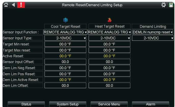
**Sensor Input Function:** Choose between HMI(None), Remote Analog Target (Input 6), or BAS Target (0-10).
