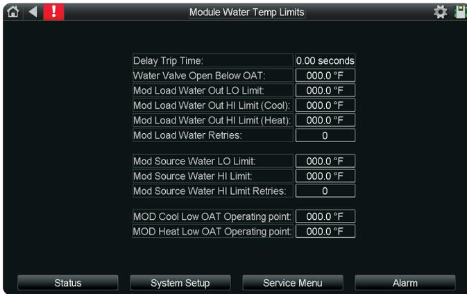
**Delay Time Trip:** The time in seconds that the module delays before triggering a freeze protection alarm.
