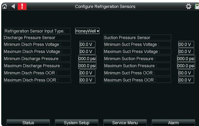
**Refrigeration Sensor Input Type:** Choose between Honeywell, Carel(default) or Custom. If Custom is selected, the below values must be set.
