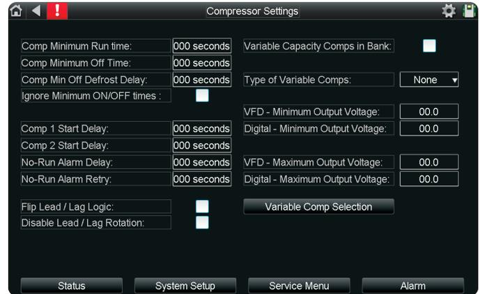
**Compressor (1/2) Start Delay:** The delay in seconds before a module compressor runs after being requested. This option typically requires no adjustment. *Default 90 sec for Comp 1 and 220 for Comp 2.*
