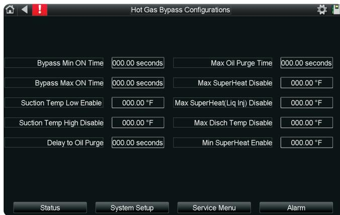
**Bypass Min ON Time:** The minimum time hot gas bypass is open.
