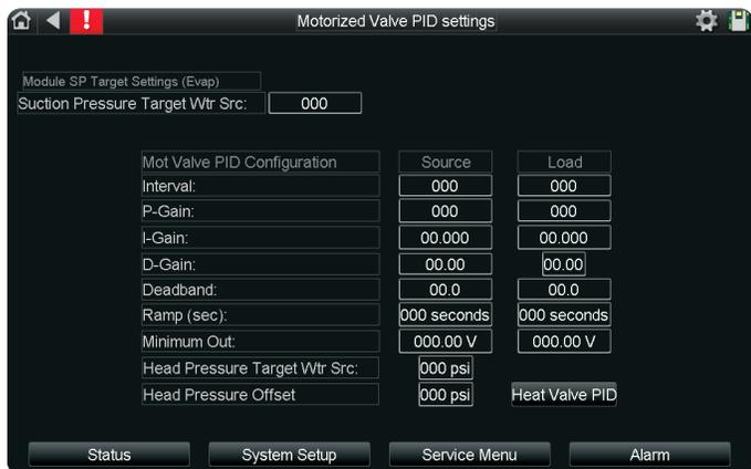
**Module SP Target Settings:** The Suction Pressure valve control target for water-source units.
