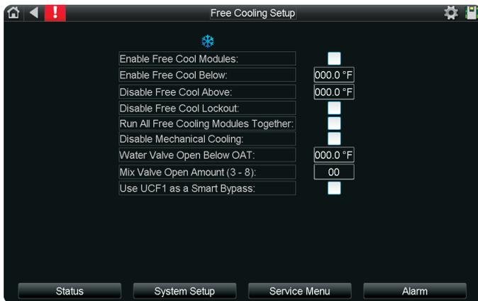
**Enable Free Cool Modules:** Enable Free Cooling if Free Cooling modules are available.
