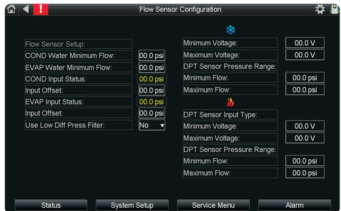
**COND Water Minimum Flow:** The minimum flow psi on Loop 2.
