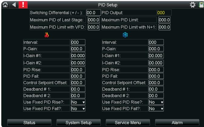
**Recommended:** Set PID tuning up to stage one compressor up/down every 5-8 minutes.
