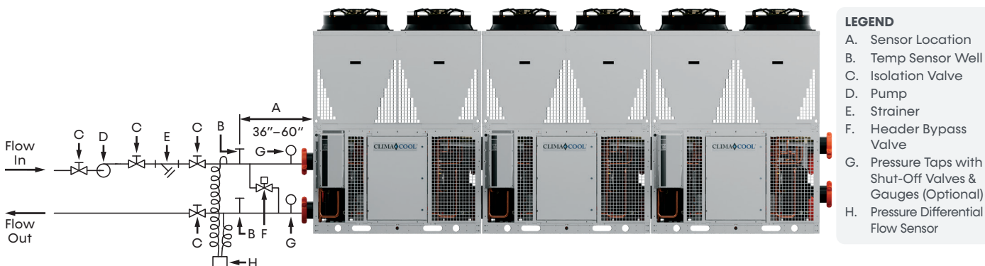
Figure 25: Field Piping Reverse Return – Preferred Piping Arrangement
