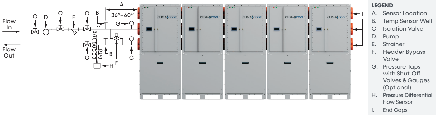
Figure 20: Field Piping Direct Return – 1 to 5 Modules
