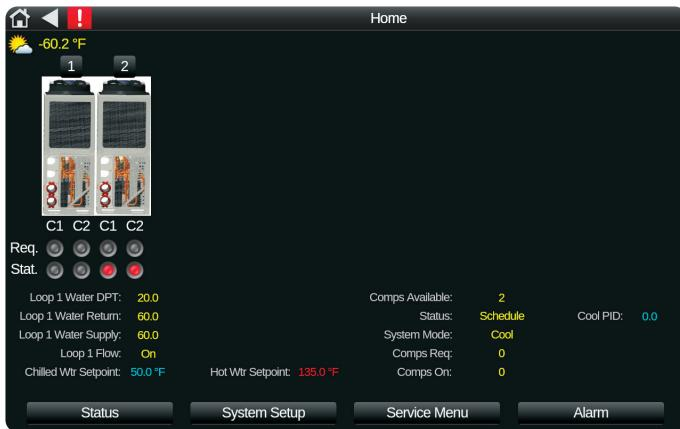
After the delay, the module status displays. After the screen times out, the display changes to the standby screen (see Figure 7).
