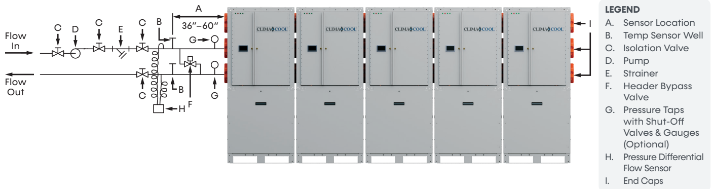
Figure 20: Field Piping Reverse Return – Preferred Piping Arrangement
